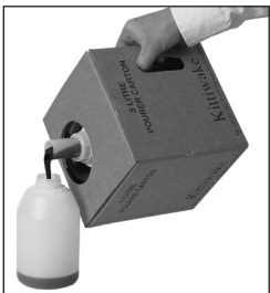
Figure 5. The full cubitainer should be placed in the pourer box and the sample transferred to the sample bottle. If more than one bottle, pour a little at a time into each one until full.
